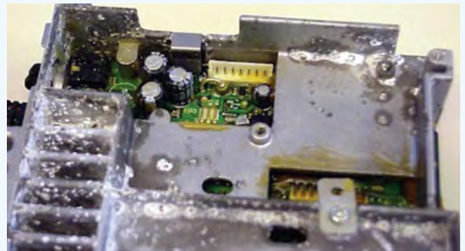
Unprotected Circuit, Heavily Corroded
